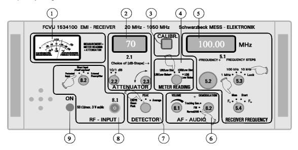
The receiver is now ready to use and frequency is tuned by rotating the encoder (5.2). The steps can be selected with (5.3).
