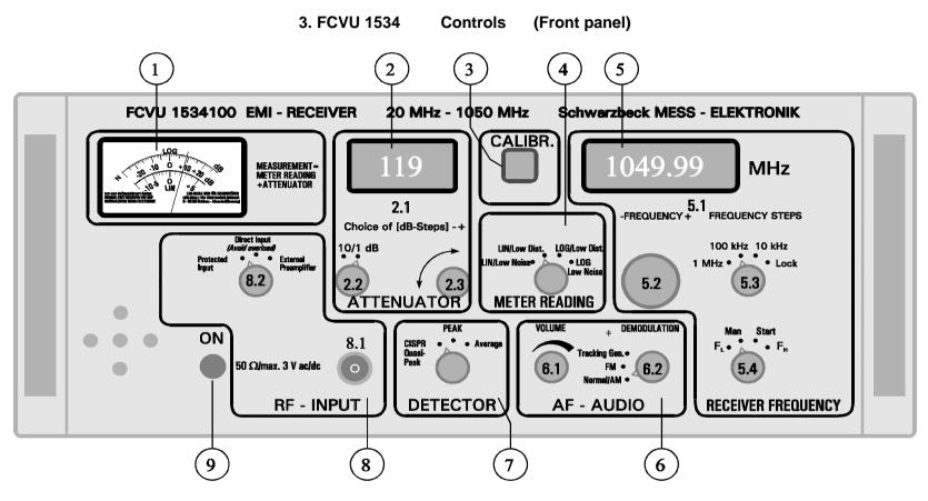
The front panel is divided into 8 areas, which unite important controls and displays. They are as follows:
